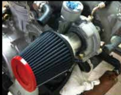
FLAME ARRESTOR #59-2040RR INSTALLED
