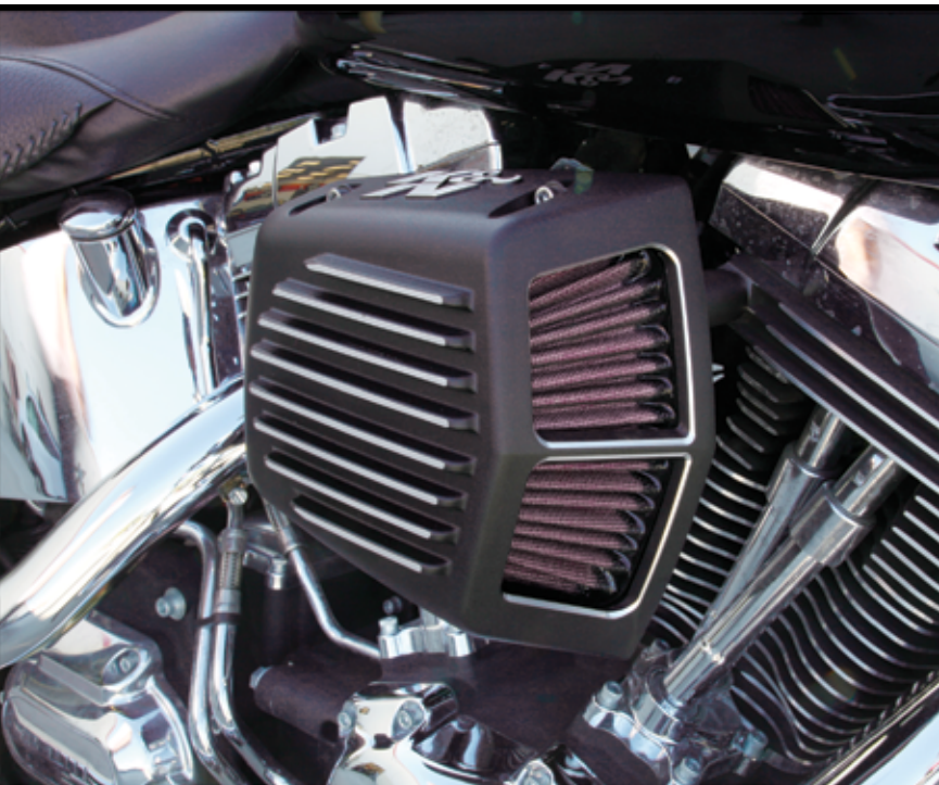
Shaker Intake System Installed
