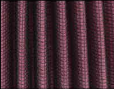
PLEATED MEDIA PROVIDES A LARGE SURFACE AREA
