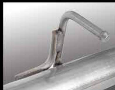
HEAVY-DUTY BRACKETS USE FACTORY ATTACHMENT POINTS
