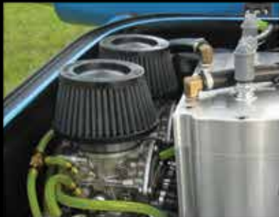
FLAME ARRESTOR #59-2046 INSTALLED
