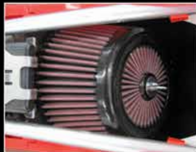
XSTREAM® SERIES AIR FILTER INSTALLED
