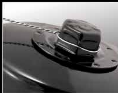
PRE-DRILLED FOR SAFETY WIRE ATTACHMENT*
