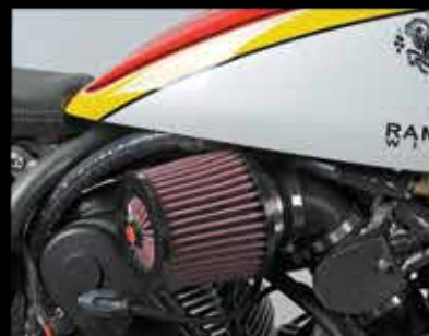
XSTREAM® SERIES AIR FILTER INSTALLED
