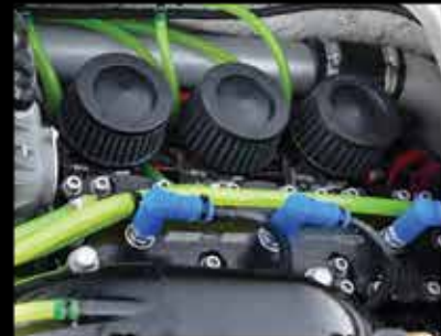
FLAME ARRESTOR #59-2045 INSTALLED
